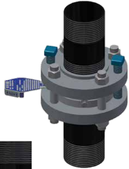
Quick-Sert installed between two ANSI (ASA) pipe flanges
